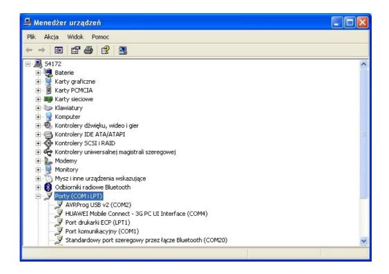
If the programmer installs at a distant COM port (it is advised to install it between COM1 and COM9). See the below picture for more details.
