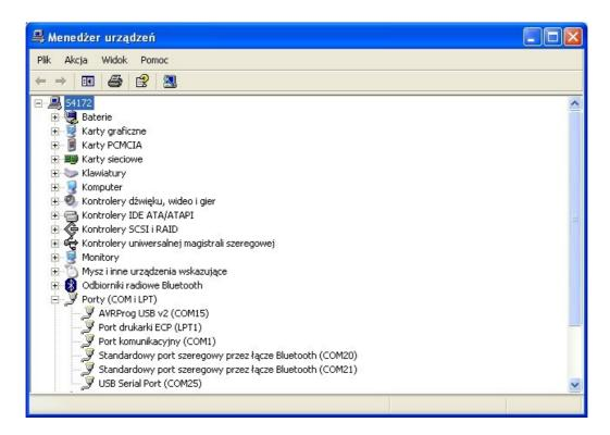
In order to change the COM port, enter programmer's advanced settings to choose a port between COM1 and COM9 (if these are already in use, try to relieve one and than check programmer's correct operation).
